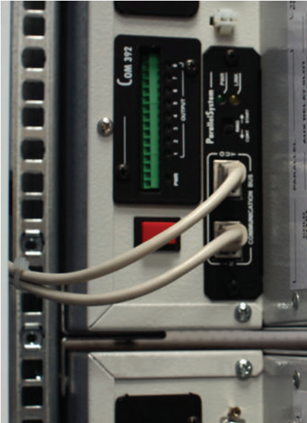
Parallel configuration and programmable relay contacts board
