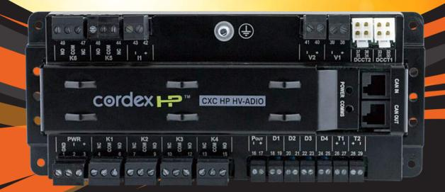
The CXC HP HV-ADIO brings advanced control and monitoring to Alpha Cordex 125/220Vdc rectifiers and systems. The HV-ADIO is part of the CXC HP series of advanced I/O peripheral incorporating flexible mounting, high accuracy, and the advanced features in the HP control platform.
